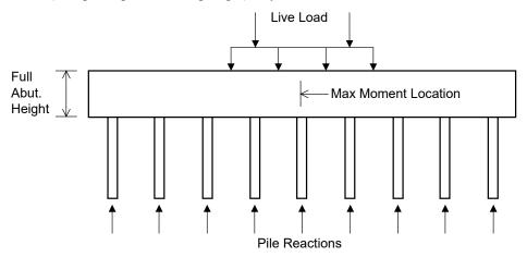
Bending of the abutment acting as a vertical cantilever below the beam seat elevation to resist soil pressures and lateral pile forces and moments for thermal expansion, and the lateral pile forces and moments only for thermal contraction.
