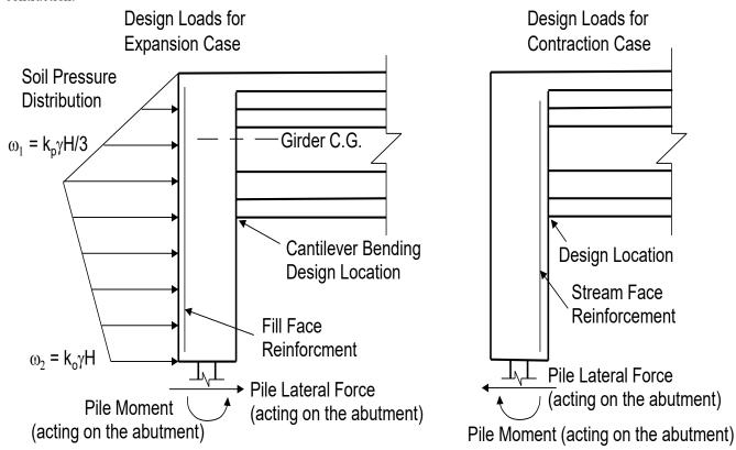
Bending of the abutment acting as a continuous beam spanning between the girders under a soil pressure load. The full section of abutment (both pile cap and end diaphragm) may be used.
